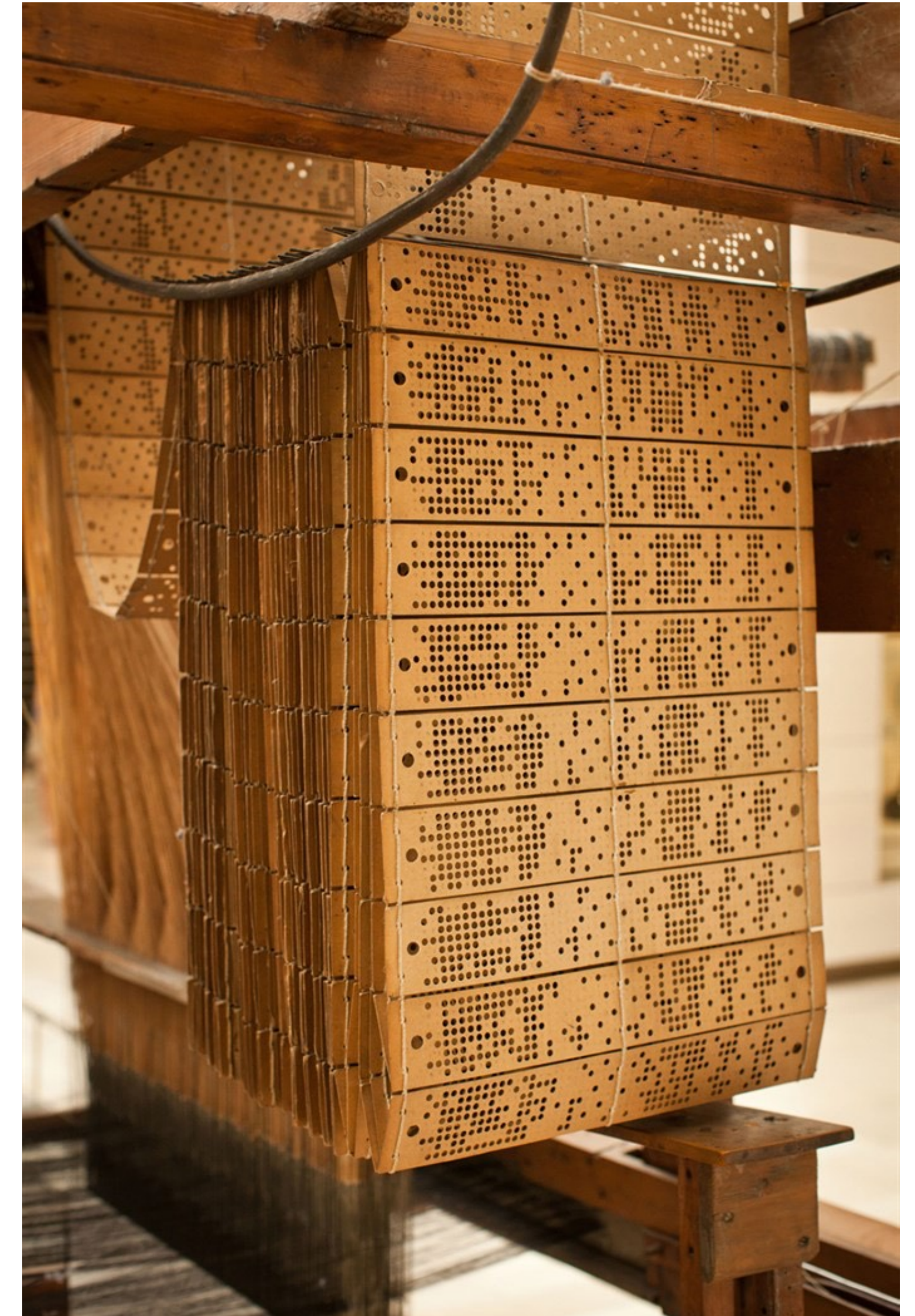
Punched cards used in a Jacquard loom
